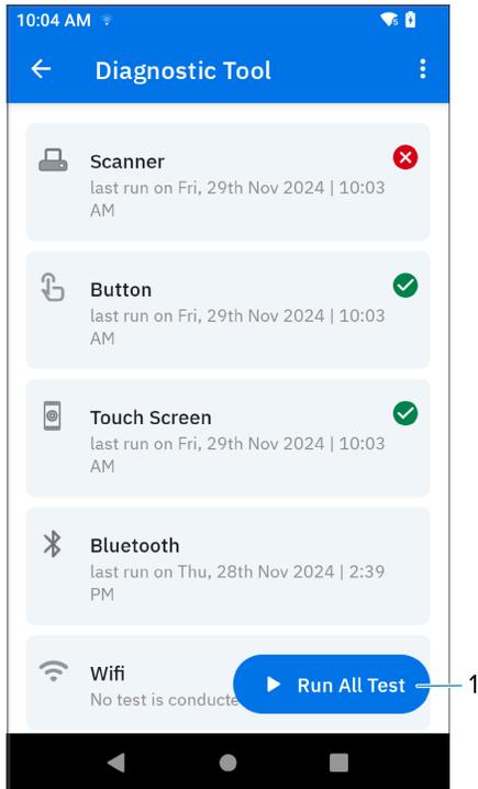
2. The **Run All Test (1)** runs all the listed tests in sequence to verify the system's health and simultaneously generates a result report.
